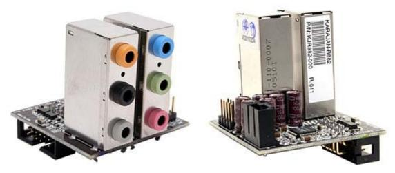
Karajan audio module: the Azalia High Definition audio Codec that is isolated on the module for improved signal-to-noise performance
