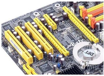
Unlike many nForce4 SLI mobos, however, the DFI RDX200 doesn't feature a paddle card for changing between single and dual graphics card modes. Instead, the switching is done via the electronics. All the user has to do is to perform the switch in the BIOS or let the BIOS detect it automatically.
