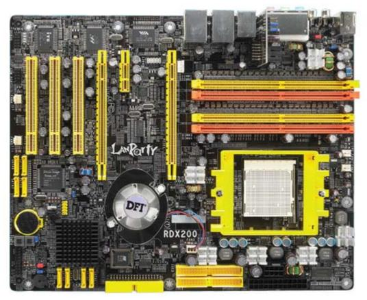
The RDX200 is built to perfection using a 6-layer PCB and high-quality components. UV sensitive (glow in the dark under dark light) slots, and a magnetic-levitation fan on the chipset heatsink make this mobo quite the looker at LAN parties as well.
